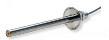
The AM3455 sensors are welded to blind flanges that can be inserted into standard tee fittings in sanitary systems using Ladish or Tri-Clover fittings.
