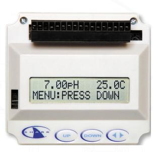
Loosen the two spring loaded screws on the front plate and a second LCD menu flips down. In addition to showing the process reading, temperature and calibration results, other menus allow the user to change input sensors (as shown below). Other menus offer diagnostics and enable the user to set relay values and fine tune parameters such as noise reduction.
