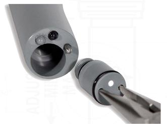
All differential probes, including the P60/65C-6 shown here feature replaceable salt bridges. The pH 7 solution in the well behind the salt bridge can also be easily replenished. Kits consisting of 3 salt bridges and pH 7 solution are readily from your Aquametrix distributor.
