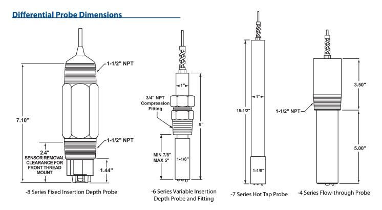
The Aquametrix family of differential probes includes the fixed insertion -8, the variable insertion -6, an extended length version of the -6 for hot tap connections—the -7 and the flow-through version -4.
