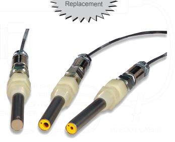
Process connections are made via a customized swage fitting with 1/2" or 3/4" NPT threads. This fitting can be screwed into a line, or tank, and it can also be turned around and connected to a standpipe for use in a submersion configuration. The AM3422 is a general purpose conductivity probe that covers a broad range of conductivities and that is ideal for harsh environments.
