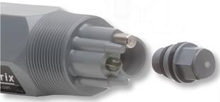
Exploded view showing the salt bridge and the well containing the reference electrode. Both the salt bridge and buffer solution can be replaced at little cost.
