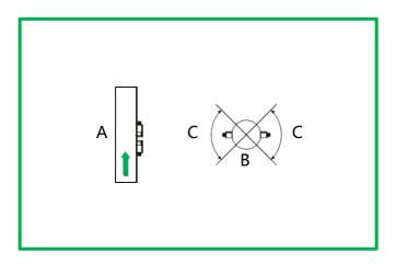
A is for an upright pipeline. Please notice that the fluid is flowing upward.
